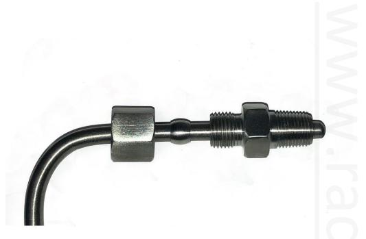
Once installed, slide the probe through the nut, then ferrule, then fitting and tighten the nut to secure the probe. Do not overtighten. In most cases, you can sink the probe until the 90 deg bend is at the fitting. This will ensure the sensing part of the probe is in the direct line of the exhaust flow.
