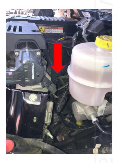
This will complete the connections of the Ultra. Turning the ignition to the "Run" position will "wake up" the Ultra. The Tuner is now ready to program the ECM. For further information on the programming process, please see our Programming manual.
